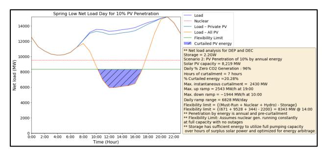
Figure 15. Low net load day with 10% PV penetration in spring when the Duke Carolinas territory is modeled with unlimited transmission capabilities
