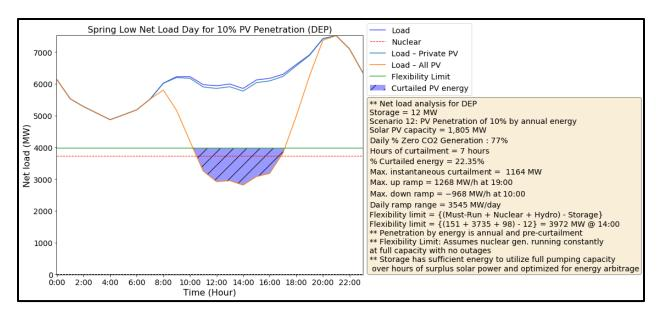
Figure 13. Low net load day for the DEP balancing authority with 10% PV penetration in spring
