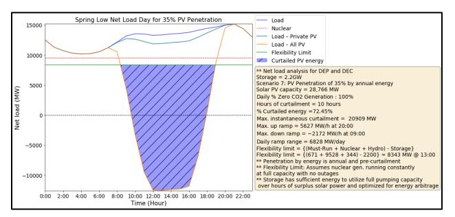
Figure 11. Minimum net load day in spring with 35% PV energy penetration
