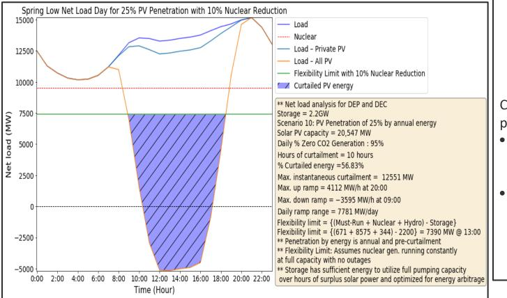
Based on 25% PV penetration case, 10% of nuclear power is retired and assumed replaced with flexible thermal generation
