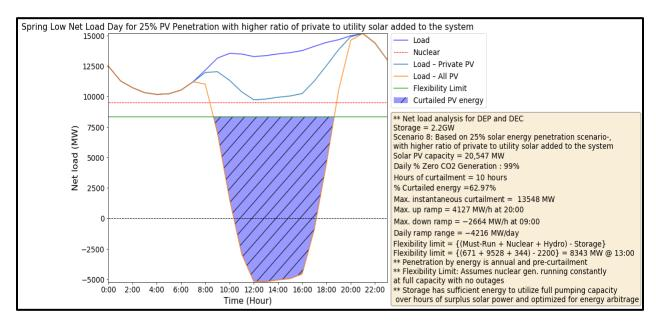
Figure 7. Minimum net load day with an increase in rooftop PV
