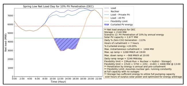
Figure 14. Low net load day for the DEC balancing authority with 10% PV penetration in spring
