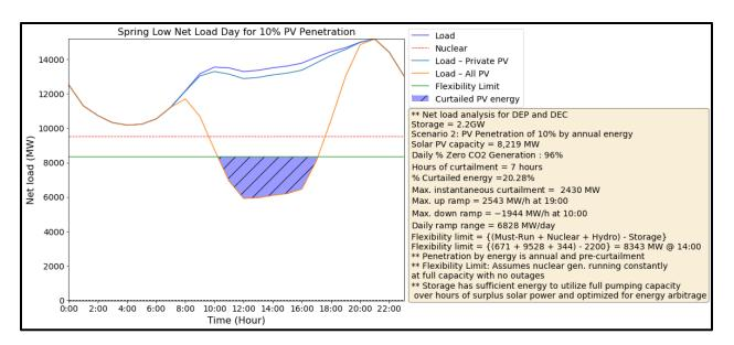
Figure 3. Minimum net load day for spring with 10% PV penetration
