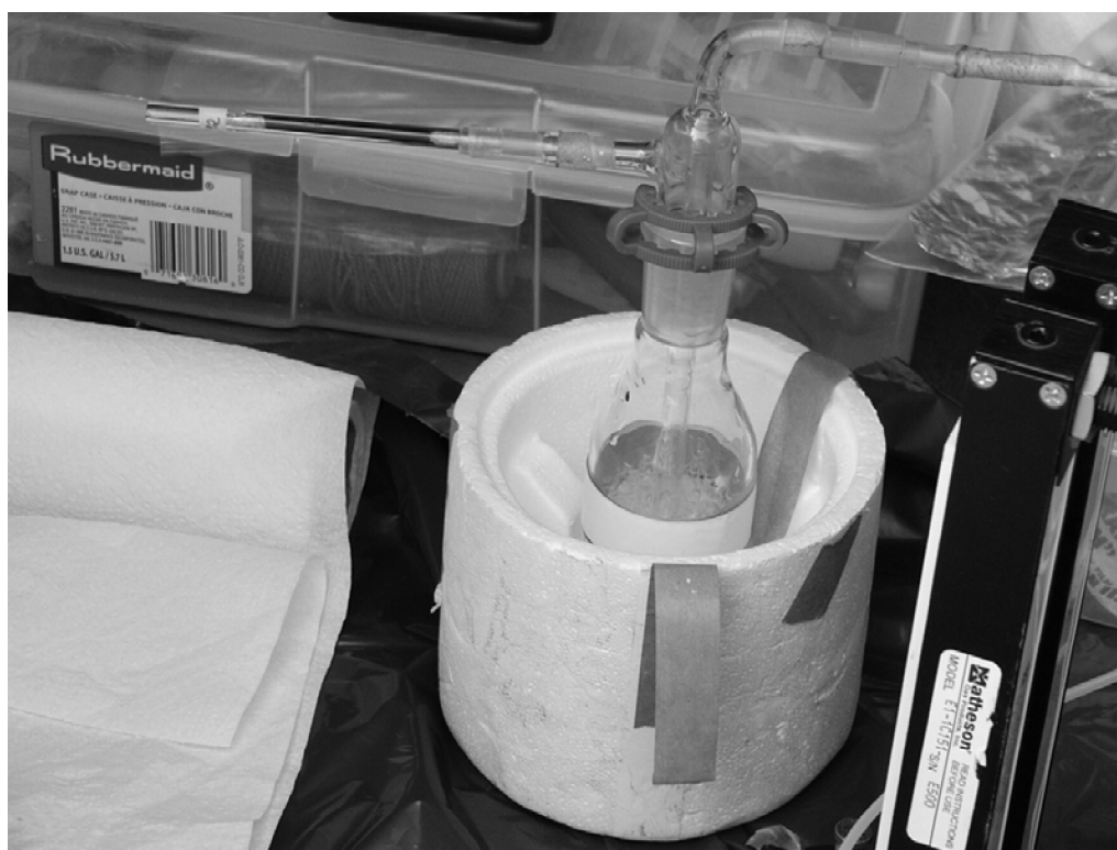
Figure 2-5 Argon Bubbling Through a Leachate Sample to Vaporize DMM
