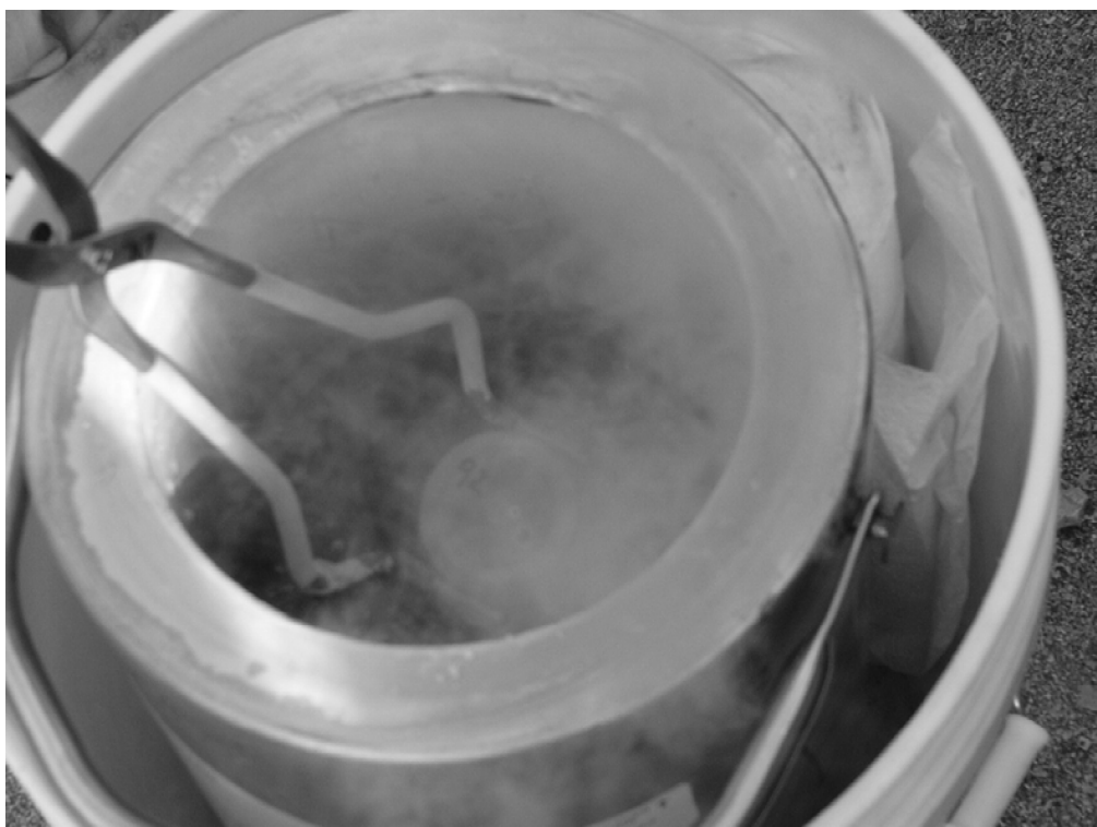
Figure 2-4 Cryofreezing a Leachate Sample in Liquid Nitrogen
