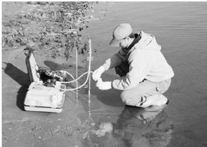
Figure 2-2 Direct-Push Sample Collection Using a T-Handled Probe
