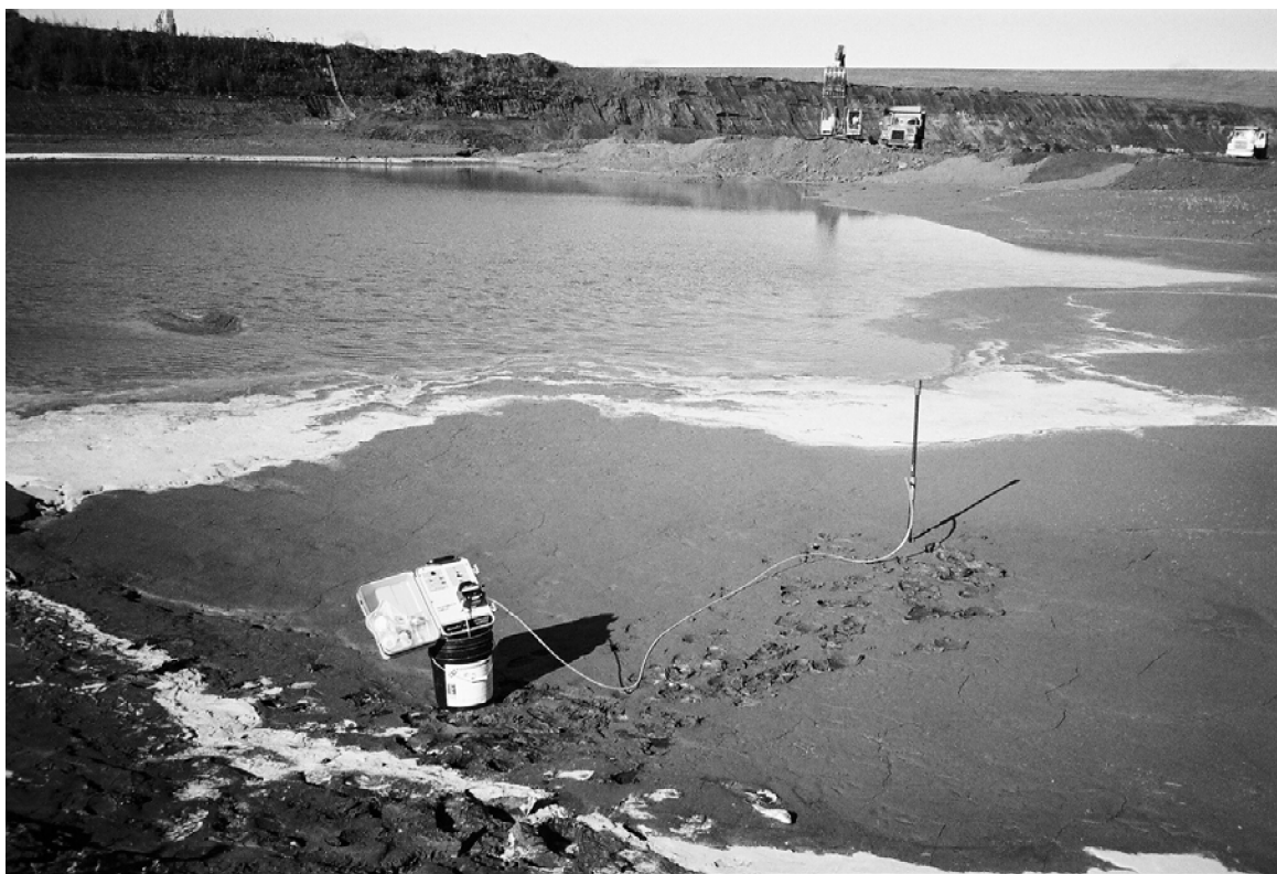
Figure 2-1 Direct Push Sample Collection Using a Drive Point Piezometer
