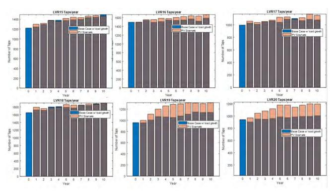
Figure 35: IEEE 123 No PV - LVR operations per year with and without PV
