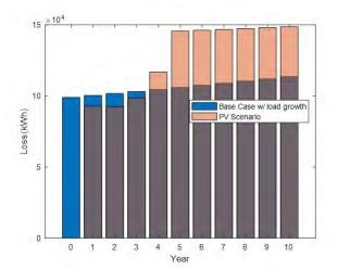
Figure 22: Yearly power loss in feeder - with and without PV
