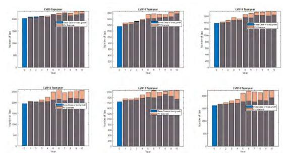
Figure 77: B03 - LVR operations per year with and without PV
