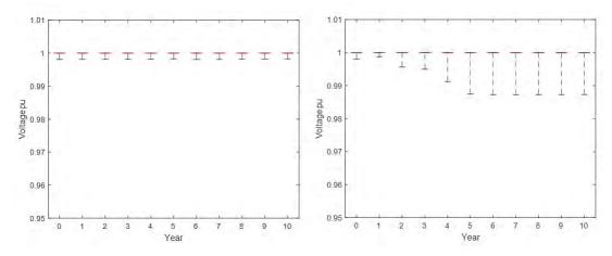
Figure 19: Minimum circuit voltage for each year of the planning period, Left: No PV, Right: with PV
