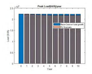
Figure 25: Yearly peak demand at substation - with and without PV
