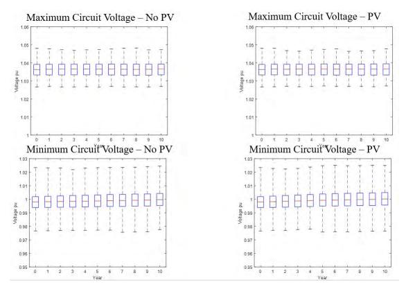
Figure 82: B03 - Voltage Statistics - with and without  $\mathrm{PV}$
