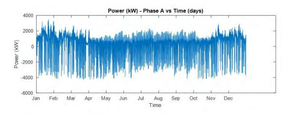
Figure 9: Net load at substation during year 10 - with PV
