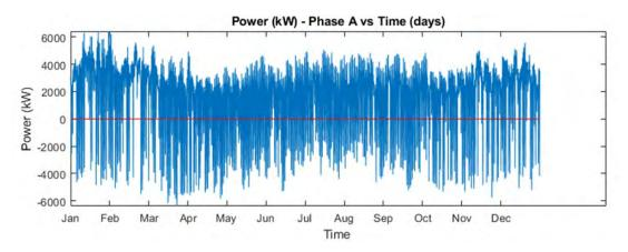
Figure 73: Net load at substation during year 10 with PV
