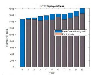
Figure 76: OLTC operations per year with and without PV
