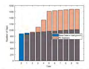
Increasing PV penetrations increases LTC operations and tapers off after year 5
