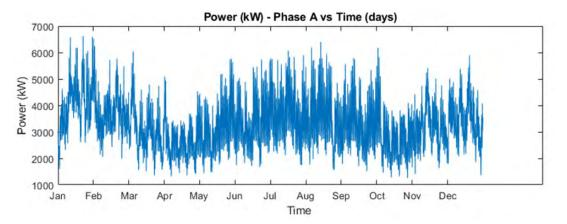
Figure 72: Net load at substation during year 10 without PV
