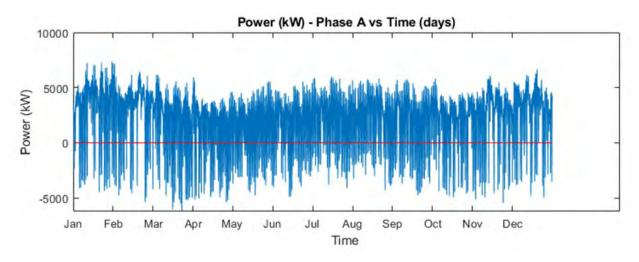
Figure 28: Net load at substation during year 10 with PV
