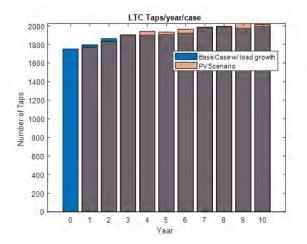
Figure 31: OLTC operations per year with and without PV
