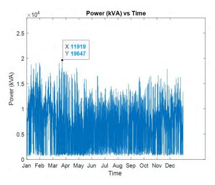
Figure 75: Net load profile year 10 - with  $\mathrm{PV}$
