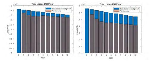
Figure 61: Total losses per year - with and without PV, Left: Total Distribution System, Right: Substation Area
