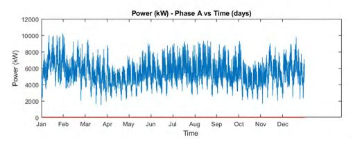
Figure 49: Net load at substation during year 10 without PV
