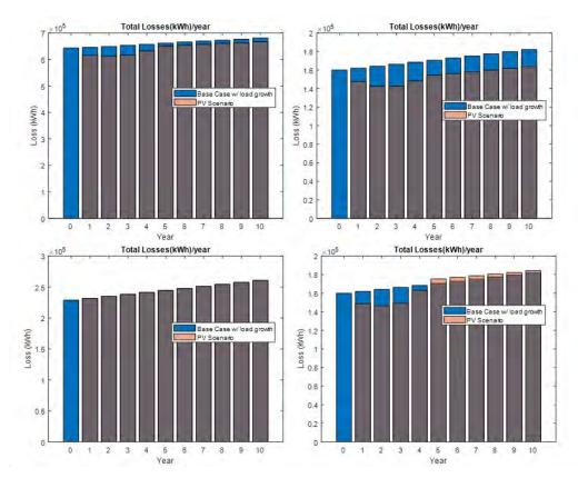
Figure 68: Feeder-wise total losses per year - with and without PV, Top Left: J1, Top Right: IEEE 123 PV1, Bottom Left: IEEE 123 No PV, Bottom Right: IEEE 123 PV2
