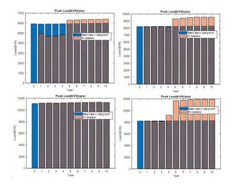
Figure 48: Feeder-wise yearly peak demand - with and without PV, Top Left: J1, Top Right: IEEE 123 PV, Bottom: IEEE 123 No PV
