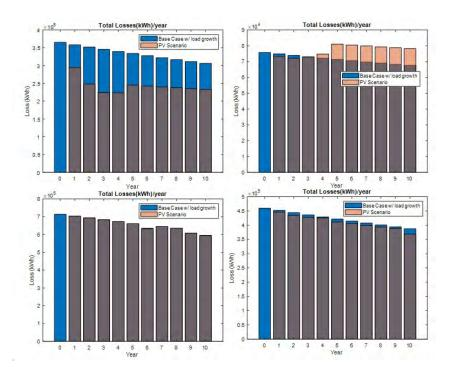
Figure 80: Feeder-wise losses per year - with and without PV, Top Left: Substation Area, Top Right: B01, Bottom Left: B02, Bottom Right: B03
