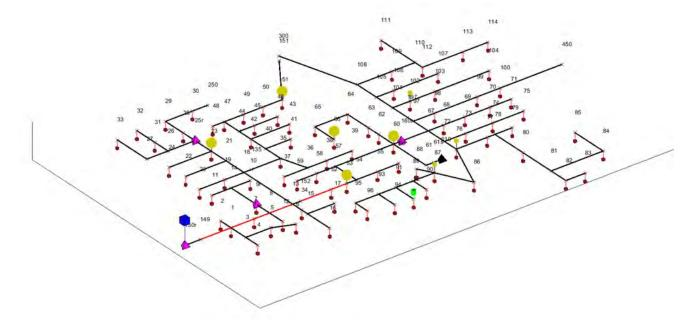
Figure 17: Equipment & line overloads in year 5 with PV
