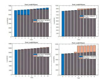
Figure 66: Feeder-wise yearly peak demand - with and without PV, Top Left: J1, Top Right: IEEE 123 PV, Bottom: IEEE 123 No PV
