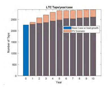
Figure 53: OLTC operations per year with and without PV
