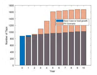
Figure 12: OLTC operations per year with and without PV
