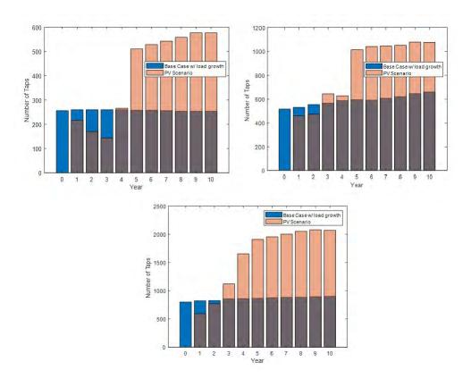
Figure 14: LVR operations per year with and without PV, Top Left: LVR 1, Top Right: LVR 2, Bottom : LVR 3
