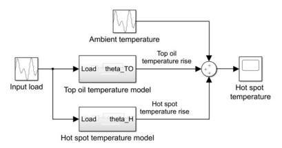
Figure A.1: Model for estimating the hot spot temperature of a transformer
