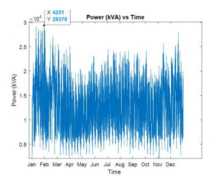
Figure 52: Net load profile year 10 - with PV
