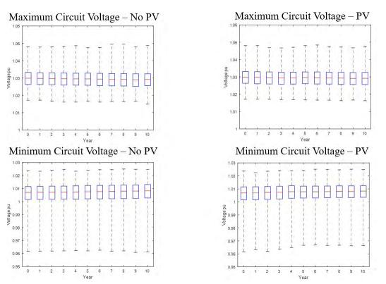
Figure 81: B01 - Voltage Statistics - with and without PV
