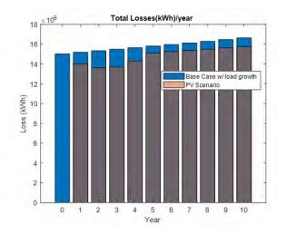
Figure 44: Total losses per year - with and without PV
