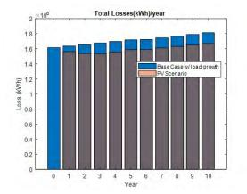
Figure 86: Total losses per year - with and without PV
