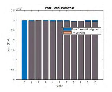
Figure 47: Yearly peak demand at substation - with and without PV
