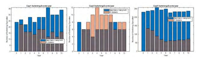
Figure 59: J1 - Capacitor switching per year - with and without PV
