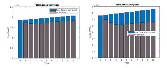
Figure 67: Distribution System Total losses per year - with and without PV, Left: Total Distribution System, Right: Substation area
