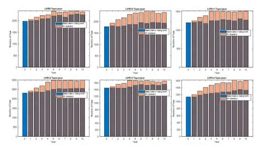
Figure 56: IEEE 123 PV1 - LVR operations per year with and without PV
