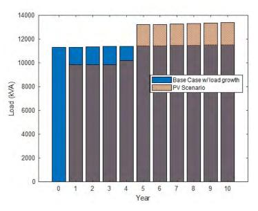
Figure 7: Yearly peak demand at the substation - with and without  $\mathrm{PV}$
