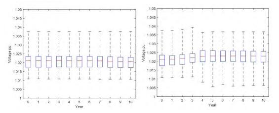
Figure 18: Maximum circuit voltage for each year of the planning period, Left: No PV, Right: with PV
