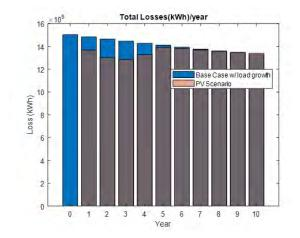
Figure 38: Total distribution system losses per year - with and without PV
