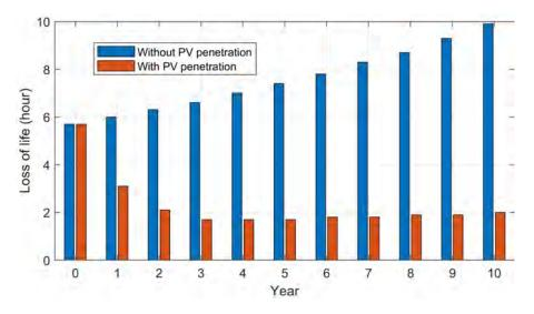
Figure 32: Comparison of transformer loss of life, with and without PV penetration
