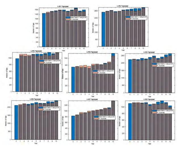
Figure 78: B02 - LVR operations per year with and without PV
