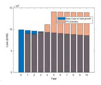
Figure 16: Total system losses per year - with and without PV
