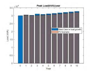
Figure 65: Yearly peak demand at substation - with and without PV
