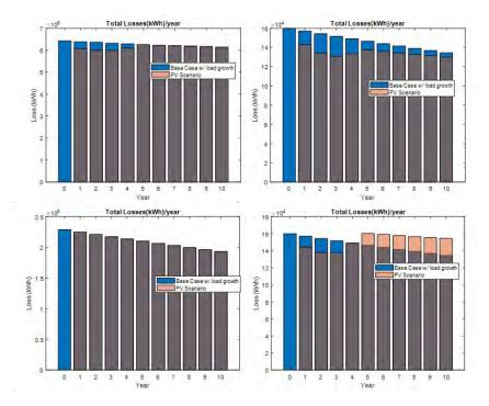
Figure 62: Feeder-wise losses per year - with and without PV, Top Left: J1, Top Right: IEEE 123 PV1, Bottom Left: IEEE 123 No PV, Bottom Right: IEEE 123 PV2
