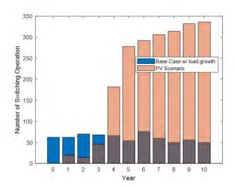
Figure 15: Capacitor switching per year - with and without PV
