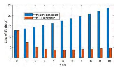
Figure 54: Comparison of transformer loss of live, with and without PV penetration
