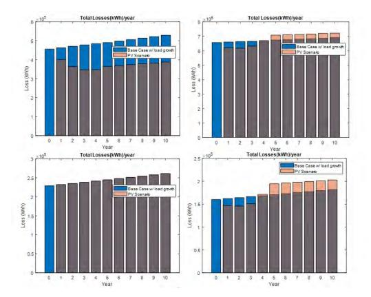
Figure 45: Feeder-wise total losses per year - with and without PV, Top Left: Substation, Top Right: J1, Bottom Left: IEEE 123 No PV, Bottom Right: IEEE 123 PV
