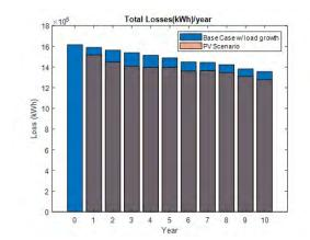
Figure 79: Total distribution system losses per year - with and without PV
